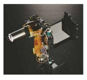
the shutter, mirror, and aperture independently. As a result, shutter release can be operated with mirror-up position during live view. Because mirror-down movement is not required, you can expect even quieter still live view shooting. And as power aperture control operates via the stepping motor, the sound of mechanical adjustment is reduced for quieter and smoother control.
